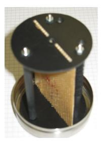
The inner structure is based on circular plastic plates that are attached to three cylindrical rods. The rods are also made of stainless steel, and are composed of smaller screw-together rods. The rods will be covered in plastic tape for isolation. Two rectangular slits on each of the plates, and a fitting contour of the circuit board, keeps the circuit board in place. The rods do not make contact with the circuit board.
