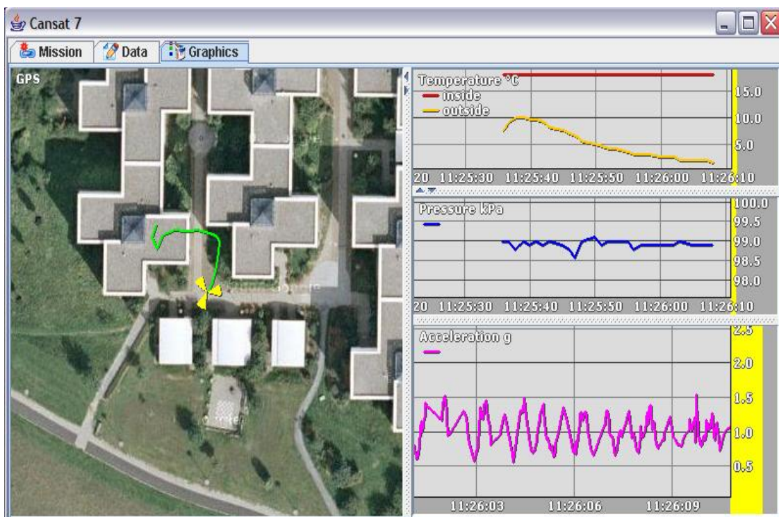
Screen shot of Cansat 7 right after the launch of the mission. The GUI shows the difference in reading from temp sensors.
