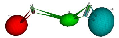
Example: The skeleton depicted above serves as an example throughout the document. The skeleton consists of 3 bodies and n = 2 hinges. Using the indexing as in the graphics, the topology is encoded by
