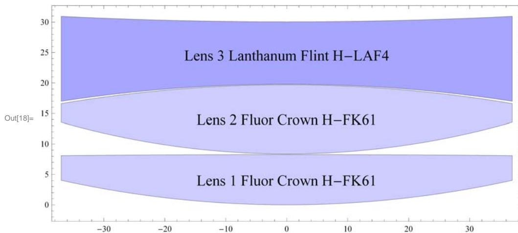
The light enters the midpoint of the surface of the first lens at coordinate (0, 0).
